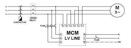
Connection diagram for low voltage line driven motors with current transformers (with nominal current above 5A & MCM LV Line):
