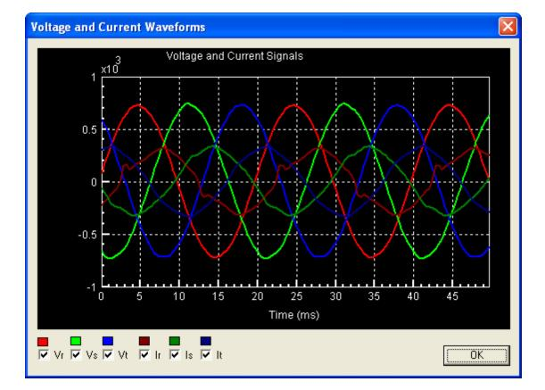
You can turn off any of the waveforms you do not wish to see by disabling the appropriate checkbox next to the label indicating this waveform.
