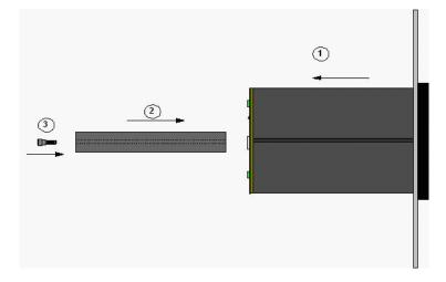
MCM has been designed to mount directly onto the front panel of the motor switchgear cabinet. Any other usage is not recommended due to the lethal voltages present at the terminals. To mount, insert the MCM unit into the prepared 91x91 mm cutout on the cabinet panel and push until the front of the unit is flush with the panel. Insert the side retainers and tighten the thumbscrews on each retainer until the MCM unit is held securely in place.
