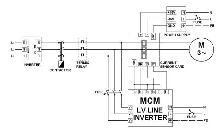
Connection diagram for low current (6 - 200A), low voltage, inverter driven motors (LEM Sensor & MCM LV Inverter):
