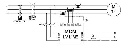
Connection diagram for low current (1 - 5A), low voltage, inverter driven motors (MCM LV Inverter):
